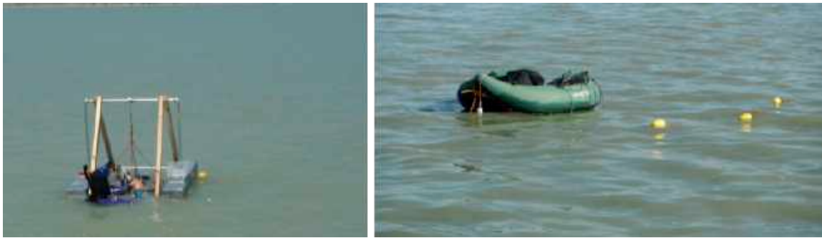
Fig. 23. SOD chamber deployment barge (left) and float tube used to carry the battery to power SOD chamber pumps (right)
