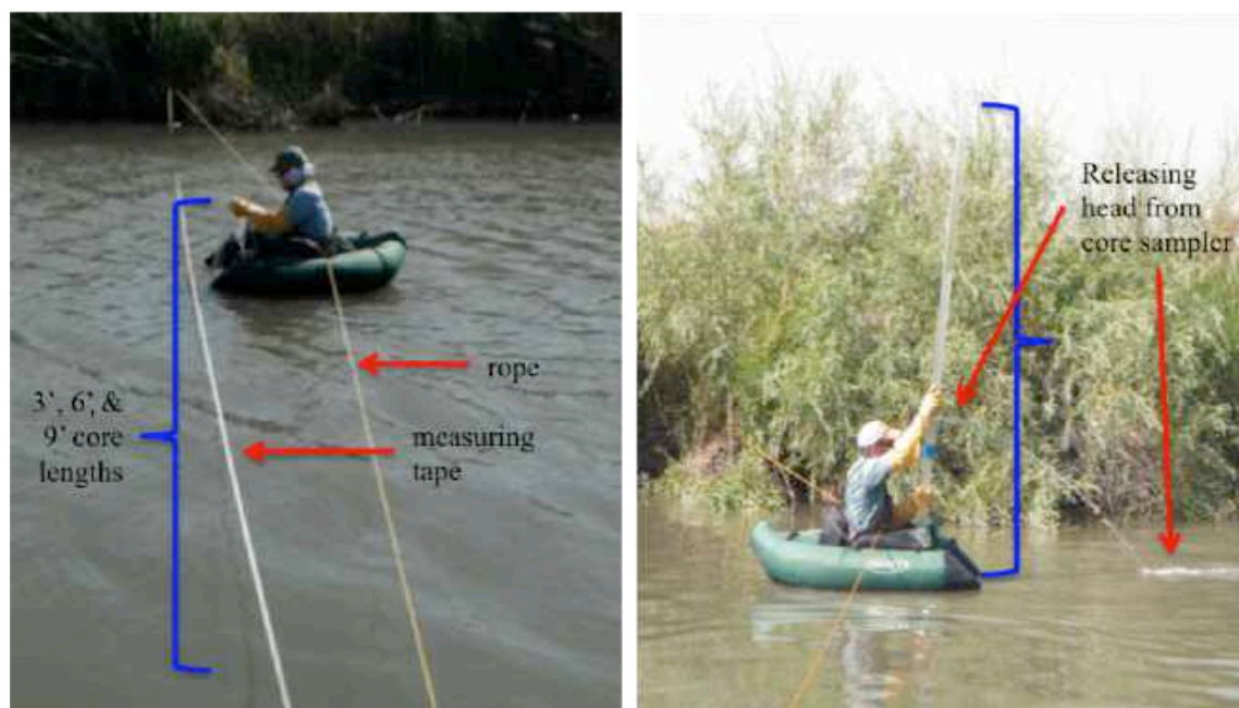
Fig. 33. Midriver sediment core sampling Note: tape measure and rope strung across river (left) and removing water from the sediment core extension (right)
