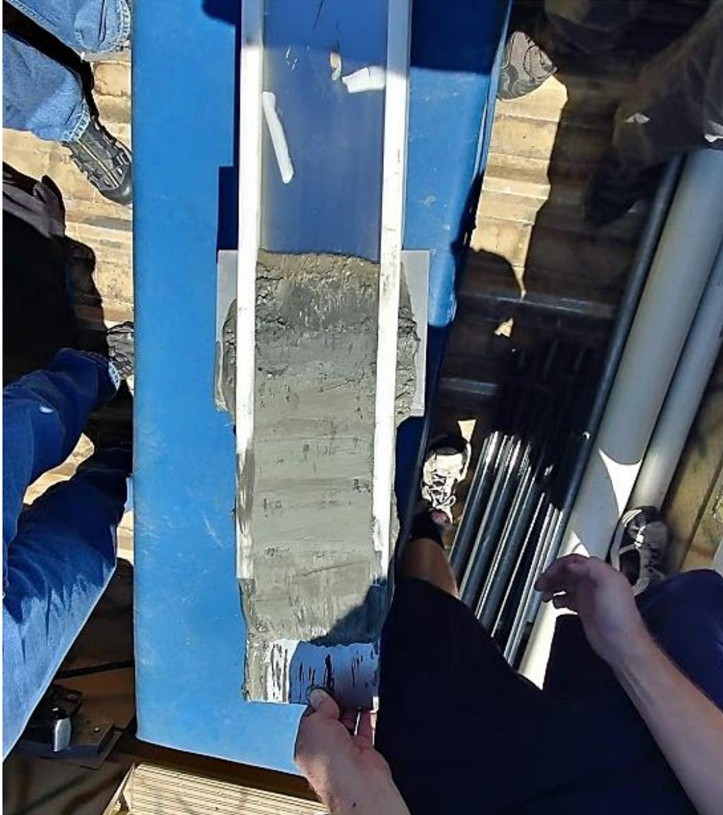
**Figure 2.** Image of the freeze core just after being removed from the bay. Laminations are clearly visible, illustrating the fact that disruption is limited by using this coring method.
