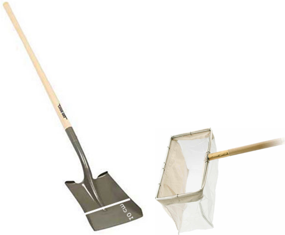
Figure 1. Shovel/net method tools. Flat-bottomed shovel with 10 cm demarcation used for scooping sediments into 4 mm mesh net.
